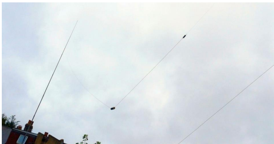
EFHW antenna: 8m vertical, 12.4m horizontal to 110uH 80m loading coil plus 2.5m extension. Works well.
