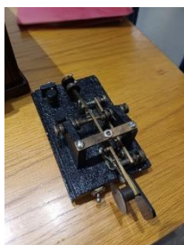
Note spring and switch on Morse Key
